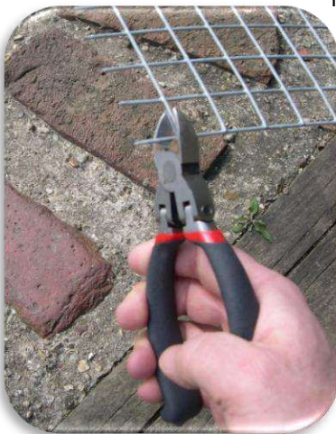
Trimming welded wire mesh with a wire cutter
