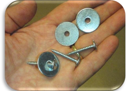
Fender washers and lath screws for attaching exclusionary mesh
